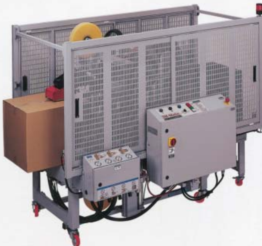
Perforated sheet metal shields allow visibility during operation and slide open for access. For safety, the 800rf will not operate with the shields open.
